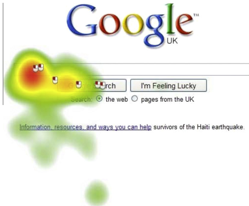
Fig. 2. Heatmap showing the relative viewing times of older participants' viewing of search page in Haiti task. Also shown are left key mouse clicks.
