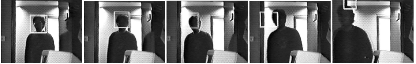
Figure 1. Five frames from a sequence in which a face was tracked using a non-adaptive model. Apparent colour changed due to different spectral composition of lighting in the corridor and the laboratory.
