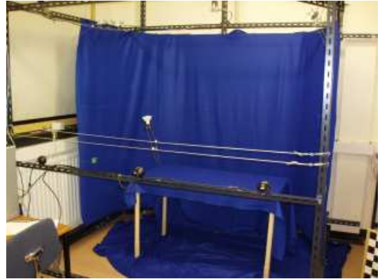
Fig. 2. Cube setup with the off-the-shelf IEEE1394 webcams used in our experiments.
