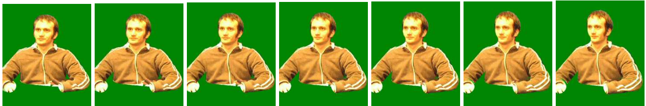
Figure 12: View synthesis with an extrapolated virtual view. The synthesised results look convincing, however, the effects of the model-based approach, such as the unrealistic shape of the head, also become obvious when extrapolating.
